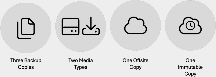
Figure 35 | Backup System with Immutable Copy
